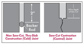
In construction (formed) joints that are not saw-cut, **Spal-Pro RS 88** should be installed at a minimum 2" depth. **DO NOT USE COMPRESSIBLE BACKER ROD IN STANDARD SAW-CUT CONTRACTION/CONTROL JOINTS!** Rod may be used 2" down in construction joints or saw-cut joints exceeding 2" in depth ONLY.
